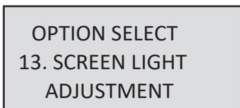
The brightness range is adjustable from 1 to 4. Default brightness value is 2. Press the UP/DOWN key to set. After successful setup, it displays “OK” for 2 seconds, then returns to the previous screen.
