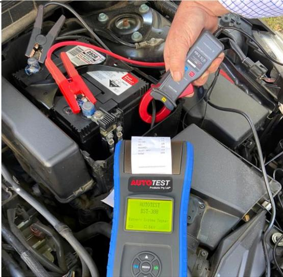
**NOTE:** (if you have the current clamp optional addition, part of the AutoTest Battery System Tester Kit.)
