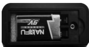
Step 2 Insert a 9V battery. There are anode and cathode marks in the battery box and also, a fixing tip. A reverse placed battery cannot be laid flat. Do not force the battery down, otherwise the battery box tip will be damaged.
