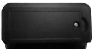
Step 3 Cover the battery box and fix the screw.
