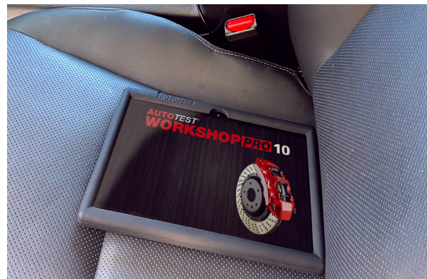
Figure 2: Workshop Pro in position ready for testing. If the unit is moving in the seat, place on the floor of the passenger seat. Supplied velcro will secure in place.
