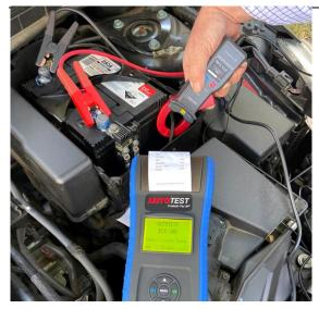
NOTE: (if you have the current clamp optional addition, part of the AutoTest Battery System Tester Kit.)
