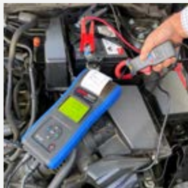
The BST-380 Battery Analyser and Current Clamp testing a car battery
