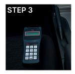
After the vehicle has come to a stop Mini Plus evaluates, and displays forward, sideways, and vertical deceleration, distance to stop and lateral deviation within the lane
