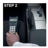
Turn on Mini Plus, accelerate the vehicle to the desired test speed (35km/hr) and apply the brakes until the vehicle is stationary.
