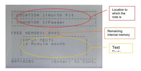
The text note will be stored in the BAM*bino*'s internal memory, it is stamped with the time and date in addition to the location and conveyor name.
