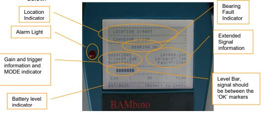
NOTE: The level bar indicates that the gain is to low, the user should increase the gain setting by pressing the up arrow (2) to increase the gain within the *OK* bands.
