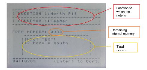
The text note will be stored in the BAM*bino*'s internal memory, it is stamped with the time and date in addition to the location and conveyor name.
