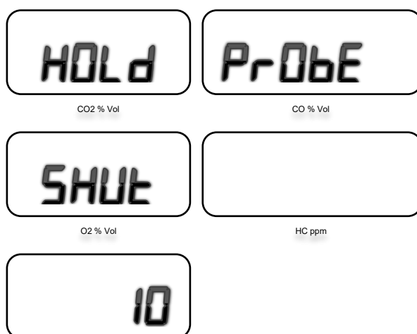
Figure 11 - Hold sampling probe shut for 10 sec.
