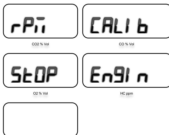
Figure 12 – RPM calibration screen, reads "RPM Calib, Stop Engine".
