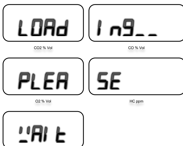
Figure 3 - Display panel while initialising hardware, reads “Loading... Please wait”.
