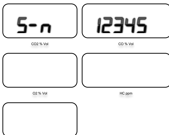
Figure 6 - Device serial no. shown at start-up, reads "S-N 12345".
