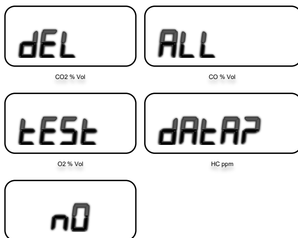
Figure 23 – “Del All Test Data?”, select Yes to clear the data or Cancel to go back.
