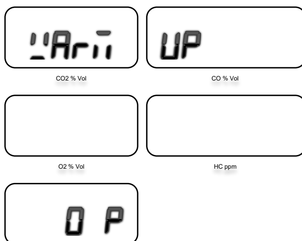
Figure 7 - Initial warm-up screen, reads "warm-up in progress 0%".
