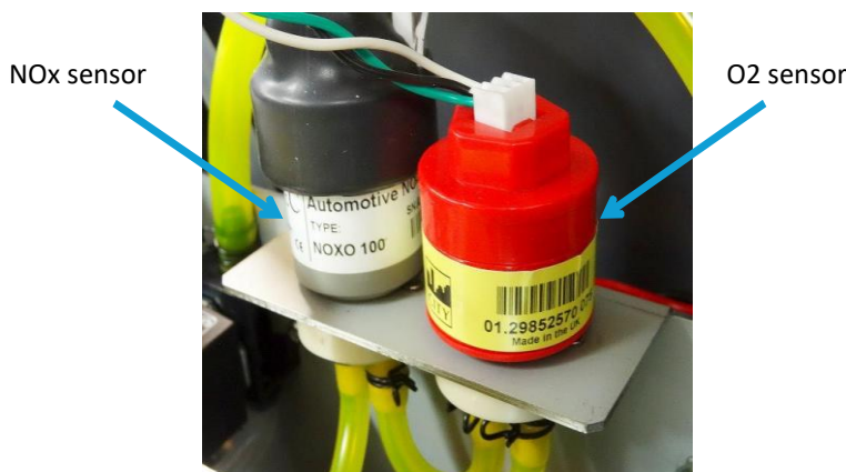
Fig. 27 NOx and O2 sensors inside the unit
