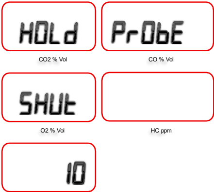
Fig. 12 Hold sampling probe shut for 10 seconds
