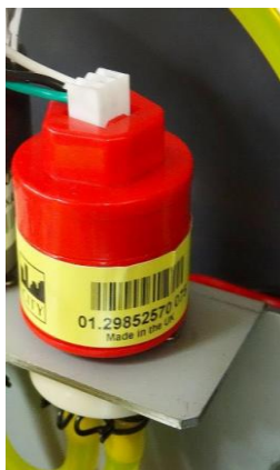
Fig. 27 O2 sensor inside the unit
