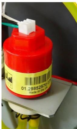
Fig. 30 O2 sensor inside the unit
