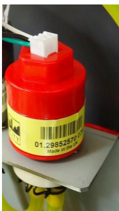
Fig. 78 O2 sensor inside the unit
