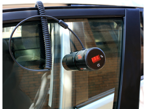
*For all door windows: The cable MUST be over the door, as pictured, for the magnets to hold. This balances the weight.
